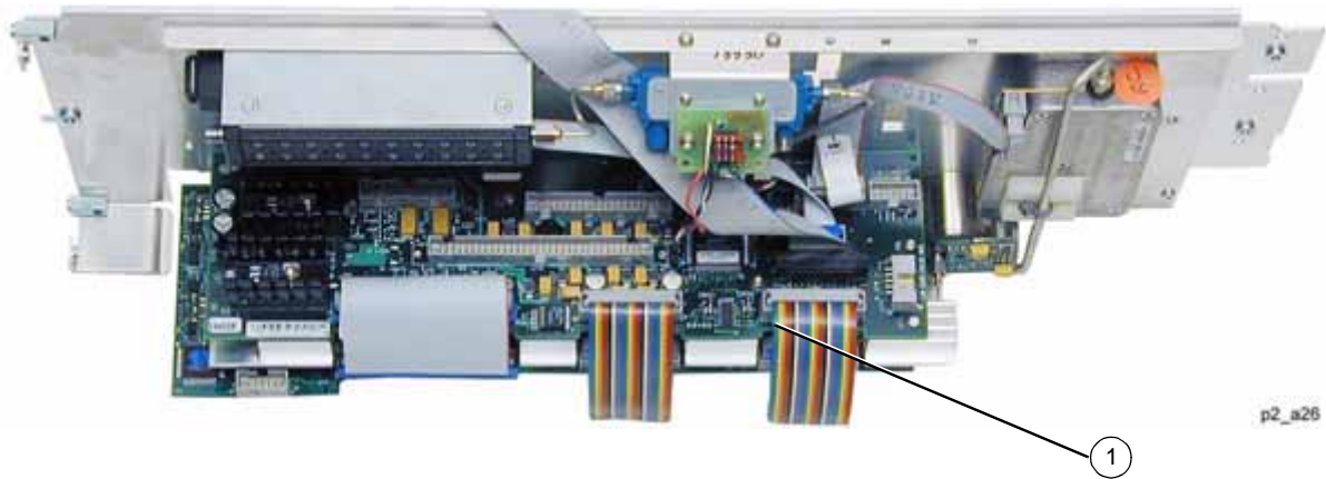
Figure 3-26 E8267D Microcircuit Interface Deck Top View
