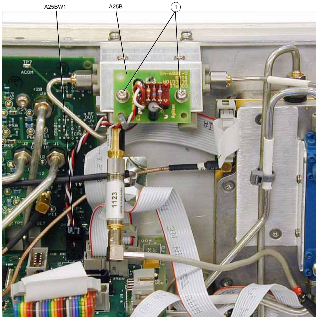
Figure 2-36 A25B Highband Detector Bias Board
